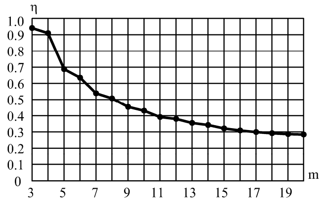
Figure 5. m -dependence of the ACID efficiency \eta for the case when the function b(y) is sinusoidal and t -dependence of the voltage u(t) has form of right-angled meander.
