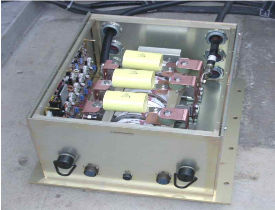
Figure 2-1 Block Switch Hardware
