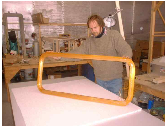
Figure 11. NbTi Superconductor Loop for Maglev 2000 Quadrupole
