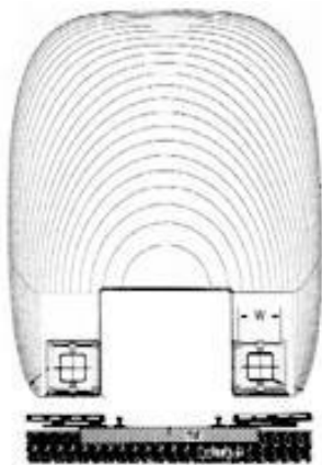
Figure 7. Drawing of levitated Maglev 2000 vehicles traveling on conventional RR track to which aluminum loop panels have been attached to the cross ties.
