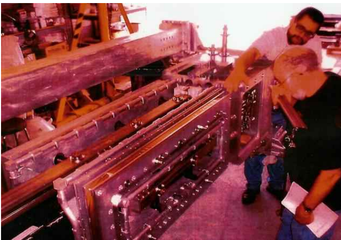
Figure 13. Assembly of Maglev 2000 Superconducting Quadrupole
