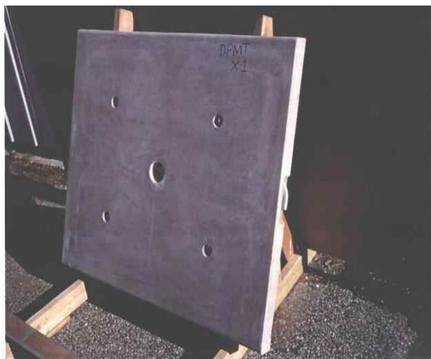
Figure 17. Polymer Concrete Panel with Enclosed Aluminum Loop Exposed for 2 Years to Outdoor Environment with Multiple Freeze-Thaw Cycles
