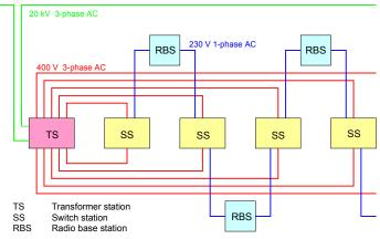
Figure 6: Radial supply of the consumers alongside the track
