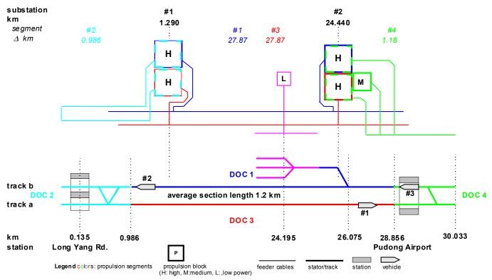
Figure 1: Propulsion layout of Transrapid Shanghai (Long Yang Road Station - Pudong Airport Line)
