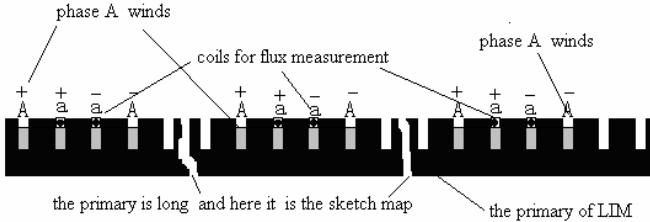
Figure 2: Mounting map for the simple measurement
