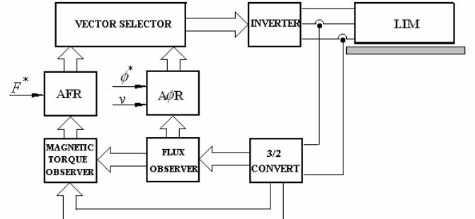
Figure 7: The ordinary control method
