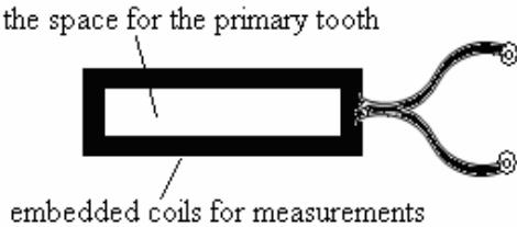
Figure 4: Structures of coils
