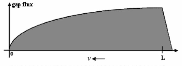
Figure 1: Gap flux distribution *the primary*
