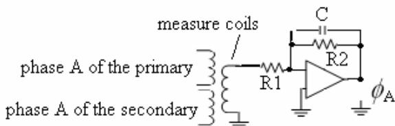
Figure 5: Integration circuits for flux
