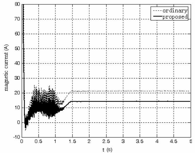
Figure 11: Magnetic current comparison between proposed and ordinary method
