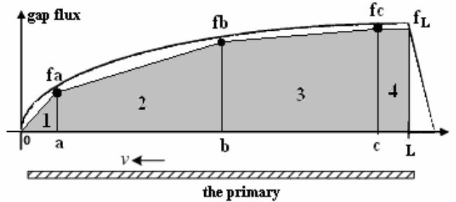
Figure 6: Gap flux approximation
