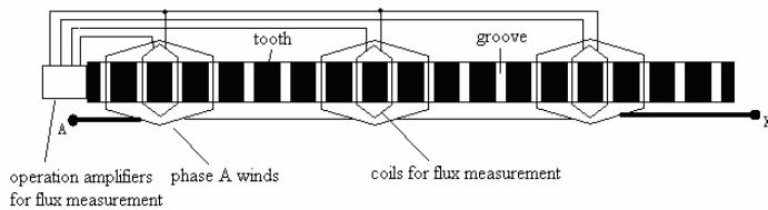
Figure 3: Lines connect coils to circuits
