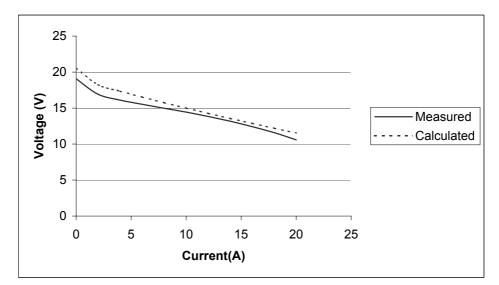
Fig 8: Comparison between experimental and calculated electrical characteristics at 45°C,  $(F_{SA}, F_{SC})=(2,5)$ , relative expander pressure references  $(H_2, air) = (1bar, 1,4bars)$ .
