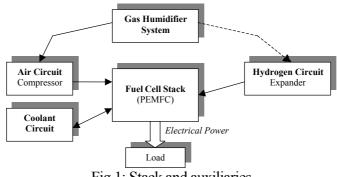
Fig.1: Stack and auxiliaries
