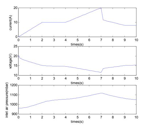
Fig 11: Simulation results for an imposed evolution of fuel cell current versus time.
