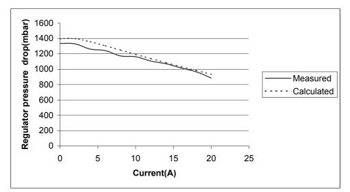
Fig 9: Comparison between experimental and calculated regulator pressure drops at 45°C, ( $F_{SA}$ ,  $F_{SC}$ )=(2,5), relative expander pressure references (H<sub>2</sub>, air) = (1bar, 1,4bars).
