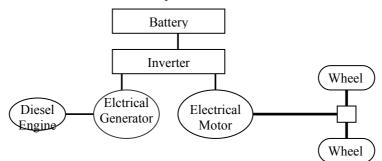
Fig. 3 Example of series hybrid vehicle
