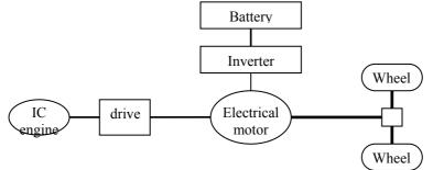
Fig. 2 Example of parallel hybrid vehicle
