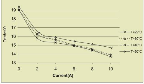
Fig 6: Static electrical characteristics for different temperatures.
