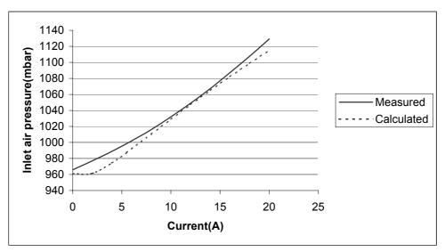
Fig 10: Comparison between experimental and simulated inlet air pressures at 45°C, ( $F_{SA}$ ,  $F_{SC}$ )=(2,5), relative expander pressure references ( $H_2$ , air) = (1bar, 1,4bars).
