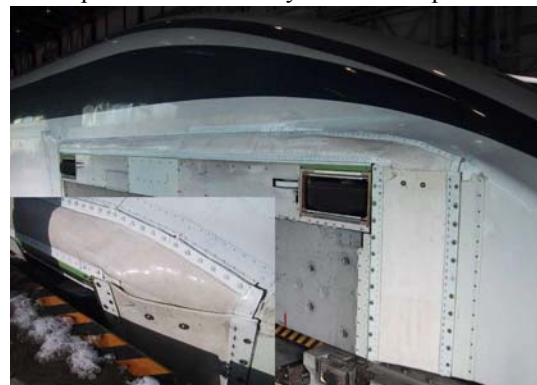
Fig. 10 Stretchable fabric fairing
